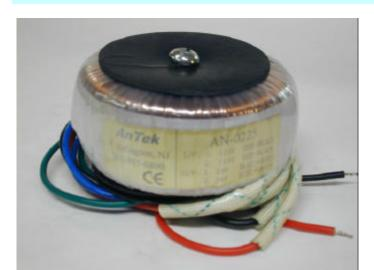
The 25VA toroidal transformers are commonly used in the noise sensitive equipment or high end audio products. They are specially designed to work on all standard 115V or 230V at 50Hz or 60Hz. These transformers have heavier gauge wires then the normal requirement to avoid the copper lost during the full power output. The dielectric test is more than 3500V in between primary and secondary coils. Please see the test data for short circuit and open circuit.
