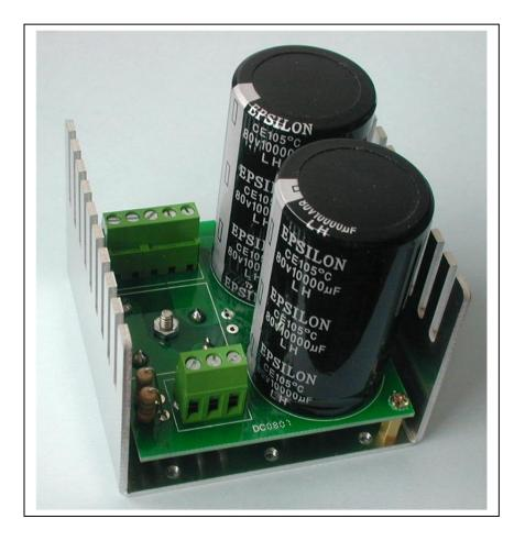
This is a complete replacement rectifier module for Antek power supplies. It includes a 50A 1000V bridge rectifier, 10000uF 80V capacitor x2, PC board, 2 connectors, 3.3K resistors x2, and aluminum heatsink housing. Assemble and tested. It can be used for up to 78Vdc 25A output power supply. Shipping weight about 1/2 pound.
