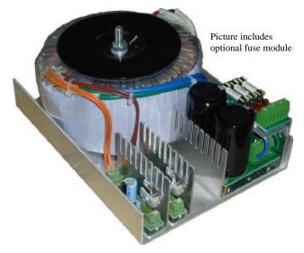
Ø 0.25" Mounting holes x4 DC output 12Vdc 1A regulated or 2A unregulated 5Vdc 1A regulated
