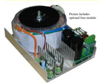
These power supplies are designed for used in the servo motor drive and high over loaded applications. They will work on both standard 115V and 230V at 50Hz or 60Hz. This toroidal transformer has heavier gauge wires then the normal requirement to avoid the copper lost during the full load output and over load output.
