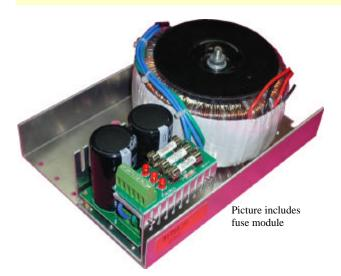
These power supplies are designed for used in the servo motor and stepper motor drive and high over loaded applications. They will work on both standard 115V and 230V at 50Hz or 60Hz. This toroidal transformer has heavier gauge wires then the normal requirement to avoid the copper lost during the full load output and over load output.
