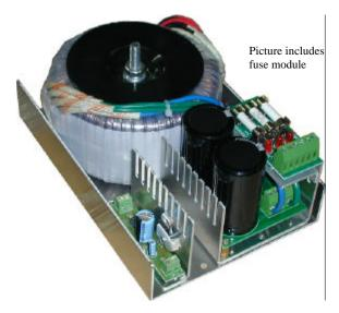
These power supplies are designed for used in the servo motor drive and high over loaded applications. They will work on both standard 115V and 230V at 50Hz or 60Hz. This toroidal transformer has heavier gauge wires then the normal requirement to avoid the copper lost during the full load output and over load output.
