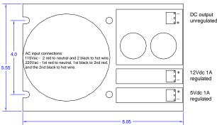
motor drive and high over loaded applications. They will work on both standard 115V and 230V at 50Hz or 60Hz. This toroidal transformer has heavier gauge wires then the normal requirement to avoid the copper lost during the full load output and over load output.
