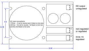
These power supplies are designed for used in the servo motor drive and high over loaded applications. They will work on both standard 115V and 230V at 50Hz or 60Hz. This toroidal transformer has heavier gauge wires then the normal requirement to avoid the copper lost during the full load output and over load output.
