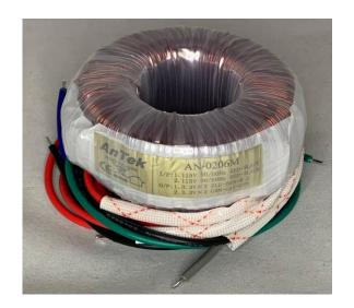
This 25VA toroidal transformer is specially designed for powering 6.3V vacuum tube filaments. It operates on standard 115V or 230V input at 50Hz or 60Hz. Built with heavier gauge copper wires than typically required, it minimizes copper loss during full power output. The transformer features extremely low magnetic leakage and exceeds 2500V in dielectric strength between the primary and secondary windings.
