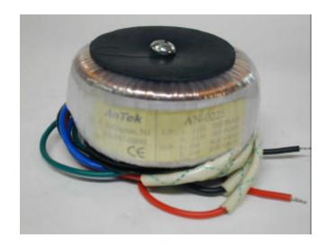
The 25VA toroidal transformers are commonly used in the noise sensitive equipment or high end audio products. They are specially designed to work on all standard 115V or 230V at 50Hz or 60Hz. These transformers have heavier gauge wires then the normal requirement to avoid the copper lost during the full power output. The dielectric test is more than 3500V in between primary and secondary coils. Please see the test data for short circuit and open circuit
