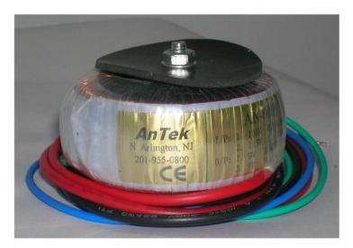
The 25VA toroidal transformers are commonly used in the noise sensitive equipment or high end audio products. They are specially designed to work on all standard 115V or 230V at 50Hz or 60Hz. These transformers have heavier gauge wires then the normal requirement to avoid the copper lost during the full power output. And it has a very low magnetic leakage. The dielectric test is more than 2500V in between primary and secondary coils.
