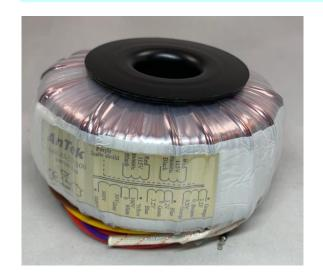
These high-performance 300VA toroidal power transformers are engineered specifically for tube audio applications. A static shield between the primary and secondary windings ensures excellent isolation and minimizes noise interference, while an external magnetic shield reduces stray magnetic fields and leakage.
