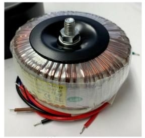
The 50VA industrial toroidal power transformer has higher efficiency than EI transformers, typically around 95 to 99%. Because of the effective containment of the magnetic flux inside the core, toroidal transformer will have a lot less interference with adjacent components. It has very lower mechanical humming and lower heat generated.
