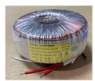
The 100VA industrial toroidal power transformer has higher efficiency than EI transformers, typically around 95 to 99%. Because of the effective containment of the magnetic flux inside the core, toroidal transformer will have a lot less interference with adjacent components. It has very lower mechanical humming and lower heat generated.
