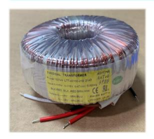
The 100VA industrial toroidal power transformer has higher efficiency than EI transformers, typically around 95 to 99%. Because of the effective containment of the magnetic flux inside the core, toroidal transformer will have a lot less interference with adjacent components. It has very lower mechanical humming and lower heat generated.
