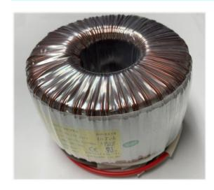
The 200VA industrial toroidal power transformer has higher efficiency than EI transformers, typically around 95 to 99%. Because of the effective containment of the magnetic flux inside the core, toroidal transformer will have a lot less interference with adjacent components. It has very lower mechanical humming and lower heat generated.
