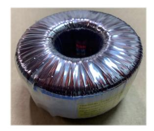
The 400VA industrial toroidal power transformer has higher efficiency than EI transformers, typically around 95 to 99%. Because of the effective containment of the magnetic flux inside the core, toroidal transformer will have a lot less interference with adjacent components. It has very lower mechanical humming and lower heat generated.
