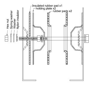
CL-500D includes 2 L bracket, 2 holding plates, 2 rubber pads, 1 insulated rubber pad, bolt, 2 hex nuts, 3 washers, insulator and 2 spring washer.
