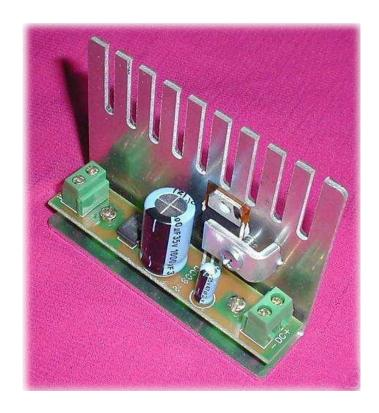
This is a small power rectifier with linear voltage regulator module for Antek power supplies. It includes all components to convert AC to DC. The aluminum housing dissipate heat generated from the voltage regulator IC (TO-220 package). For more electrical specification, please check the IC data online.
