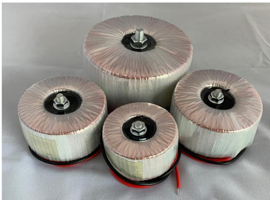
This is a newly design power filter choke with toroidal core. It allows the winding can be distributed around the whole of the core, which gives better utilization of the core material, shorter magnetic path, and further helps the Q value.
