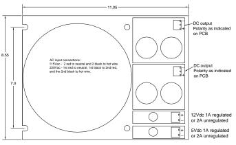
These power supplies are designed for used in the servo motor drive and high over loaded applications. They will work on both standard 115V and 230V at 50Hz or 60Hz. This toroidal transformer has heavier gauge wires then the normal requirement to avoid the copper lost during the full load output and over load output. It can easily handle up to 200% over load for few minutes.
