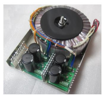
This power supply is designed for use in the stepper or servo motors and heavy load applications. It will work on both standard 115V and 230V at 50Hz or 60Hz. This toroidal transformer has heavier gauge copper wires than the normal requirement to avoid the copper loss during the full load output and over load output. Peak output current can be as high as 150% of rated current for a minute.
