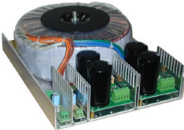
These power supplies are designed for used in the servo motor drive and high over loaded applications. They will work on both standard 115V and 230V at 50Hz or 60Hz. This toroidal transformer has heavier gauge wires then the normal requirement to avoid the copper lost during the full load output and over load output. It can easily handle up to 200% over load for few minutes.
