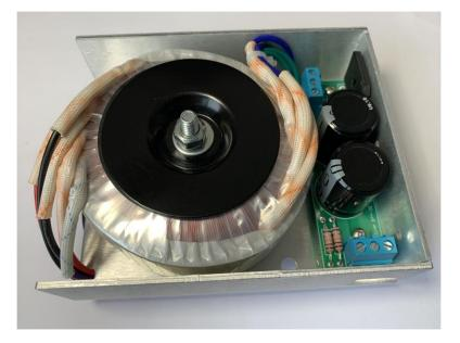
This power supply is specifically designed for small power applications and can function on both standard 115V and 230V power sources at 50Hz or 60Hz frequencies. The toroidal transformer used in this power supply has very low magnetic leakage, which prevents it from interfering with other circuits. It also has a static shield between the primary and secondary components that reduces leakage current. In addition, it is more reliable compared to switching power supplies.
