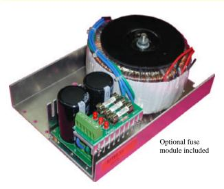
4.0 AC input connections: 15% - 2 red to returnal and 2 black to hot wire. 5.55 and the 2/rd black to hot wire. and the 2/rd black to hot wire. 8.05 These power supplies are designed for used in the servo motor and stepper motor drive and high over loaded applications. They will work on both standard 115V and 230V at 50Hz or 60Hz. This toroidal transformer has heavier gauge wires then the normal requirement to avoid the copper lost during the full load output and over load output.
