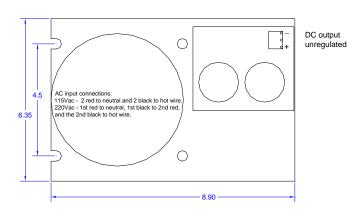
These power supplies are designed for used in the servo motor and stepper motor drive and high over loaded applications. They will work on both standard 115V and 230V at 50Hz or 60Hz. This toroidal transformer has heavier gauge wires then the normal requirement to avoid the copper lost during the full load output and over load output.
