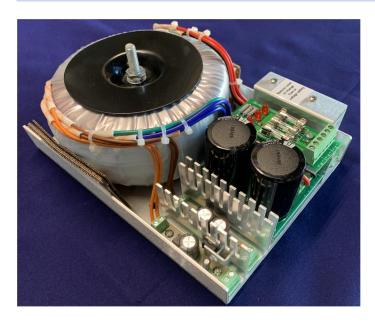
This power supply is designed for use in the stepper or servo motors and heavy load applications. It will work on both standard 115V and 230V at 50Hz or 60Hz. This toroidal transformer has heavier gauge copper wires than the normal requirement to avoid the copper loss during the full load output and over load output. Peak output current can be as high as 150% of rated current for a minute.
