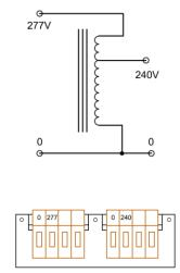
Please note: the autotransformer is not electrically isolated, as the input and output share the same winding.
