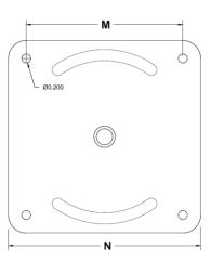
The CA-00x toroidal transformer covers are specially designed for cosmetic look and to prevent any magnetic field or electrical noise interfere with the sensitive components in equipment. This is a new economical version of CA-xxx covers.
