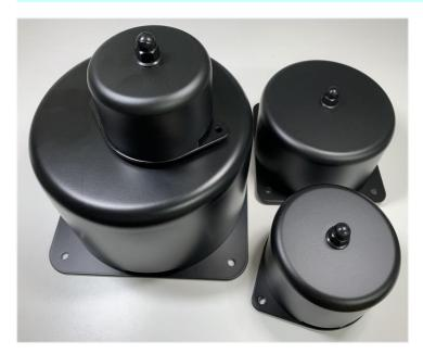
This covers are made for LK chokes, MP / MS output transformers, AN / AS / AU series power transformers and standard toroidal transformers. They were fabricated with metal spinning and stamping technique from 20 gauge steel. The whole cover is powder coat in semi-gloss black.
